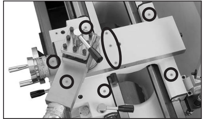
Figure 74. Location of the nine ball oilers on the carriage components.
